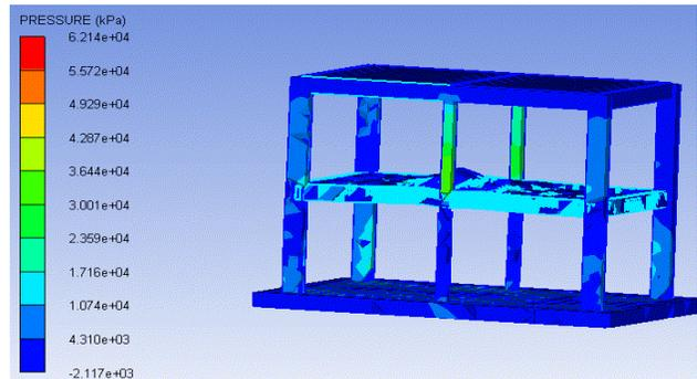
**Figure 14.** The pressure values on the elements of the building obtained from blasting analyses
