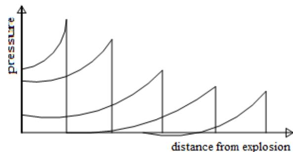
**Figure 3.** Pressure wave-distance interaction related to blasting [4]
