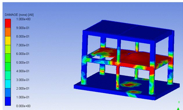
**Figure 15.** The damage ratios occurred due to blasting
