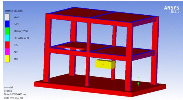
Figure 12. The place of blasting material (TNT) in the building
