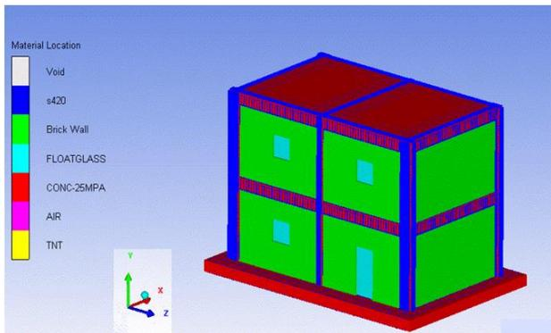
Figure 7. 3D drawing model of a two-storey reinforced concrete building
