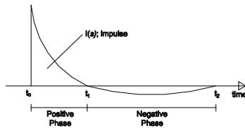
Figure 4. Pressure- Time graph of the explosion [10]
