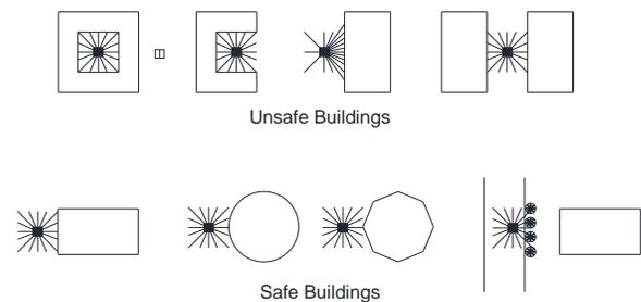
Figure 5. Safe and unsafe buildings against to blasting effects [16]
