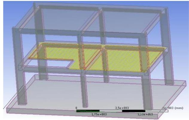
Figure 11. 3D finite element model of a two-storey reinforced concrete building
