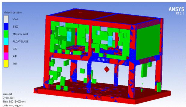
**Figure13.** Deformed shape of the two-storey building after explosion
