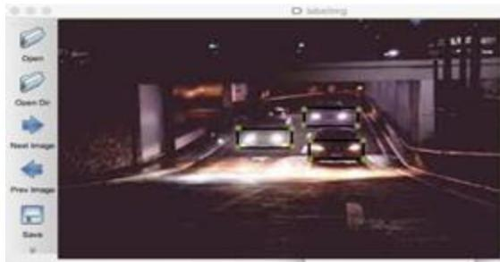
Fig.3. Labelling application vehicle headlight tagging
