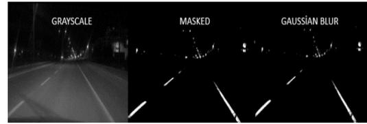
Fig.15. Steps of image filtering
