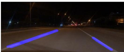
Fig.21. Detection of lane lines
