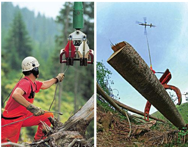
Figure 2. The hooker attaching chokers to the lifting cable attached with double load-hooks (left) and helicopter grapple (right) (URL-2)
