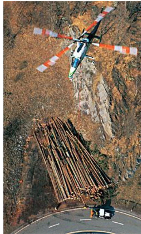
Figure 3. Placing logs at the landing (URL-2)
