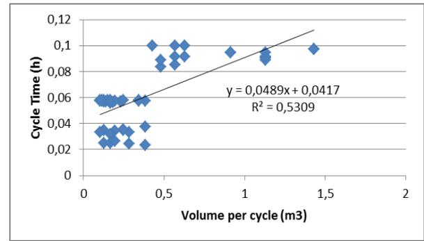
Figure 5. Effect of volume per cycle on cycle time
