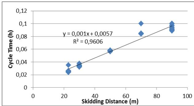
Figure 4. Effect of skidding distance on cycle time
