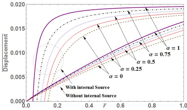
Figure 9. Variation of displacement  $\bar{u}_r$  along the  $\bar{r}$  direction for different  $\alpha$ .
