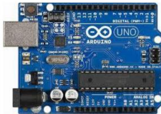
Figure 2. Arduino Uno microcontroller development board [10]
