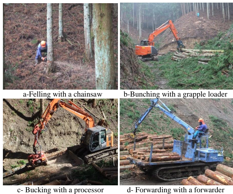
Figure 2. The stages of mechanized logging operation
