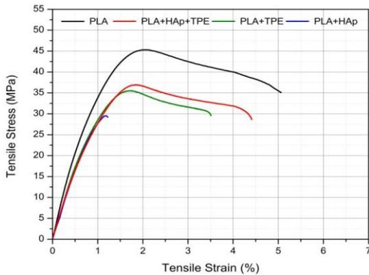
**Figure 6.** Tensile stress- strain behavior of 3D printed tensile test specimens.
