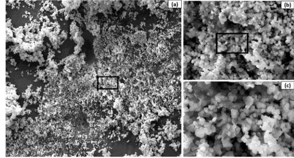
**Figure 1.** SEM (a) 500x, (b) 1000x and (c) 20000x magnifications of HAp powders.
