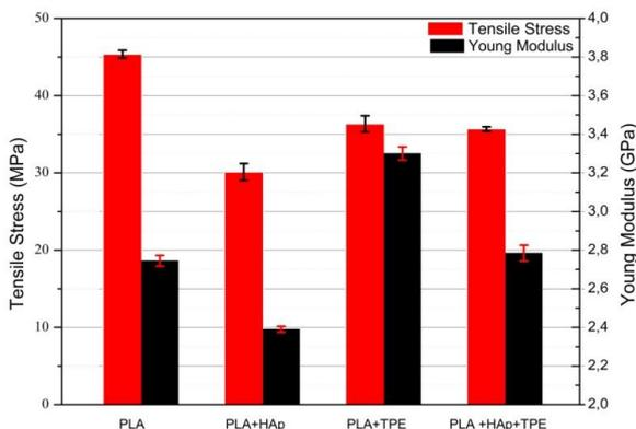
**Figure 7.** Tensile strength and Young modulus of 3D printed tensile test specimens.
