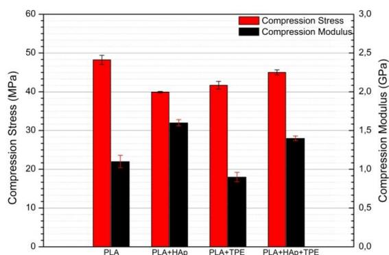
**Figure 9.** Compression strength and compression modulus of 3D printed compression test specimens.
