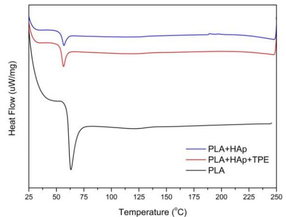
Figure 5. Heat Flow – Temperature of PLA and PLA-HAp composites.
