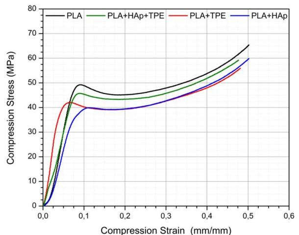
**Figure 8.** Compression stress- strain behavior of 3D printed compression test specimens.
