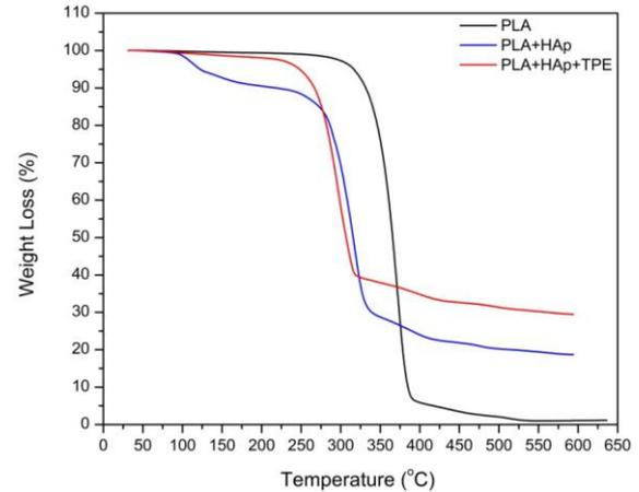
Figure 4. TGA thermogram graph of PLA and PLA-HAp composites.
