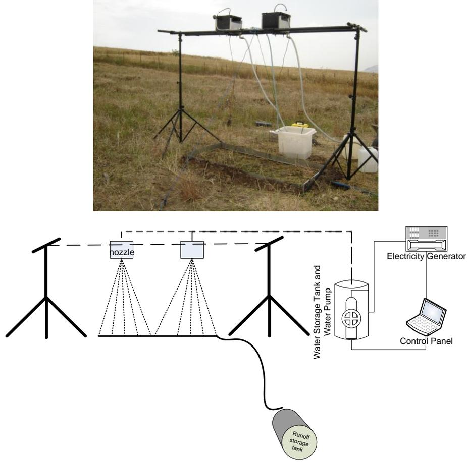
Figure 2. Schematic view of the BSTF1. Above, the actual device established in the lab and below, the general structure of the BSTF1
