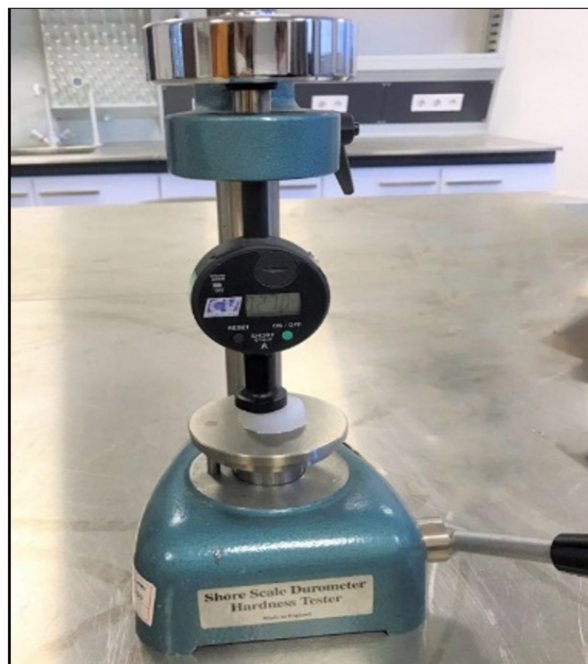
Figure 4. Hardness measurement with shore a tester
