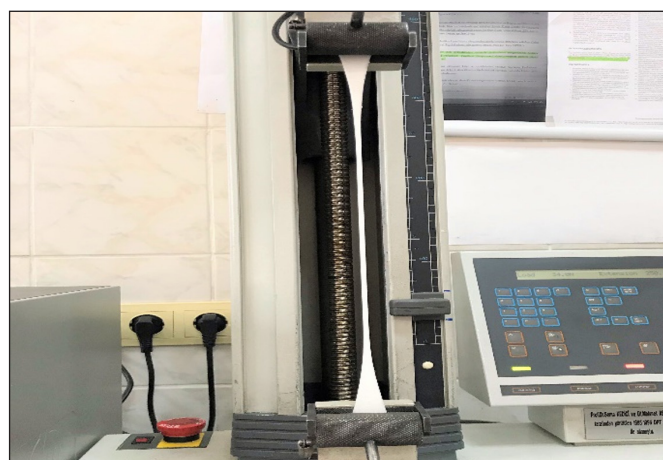
Figure 2. Tensile strength and elongation percentage test
