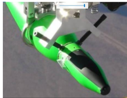
Figure 1. 81 mm Precision Air-Dropped Guided Mortar (ADM) with Two Fins-General Dynamics [28]
