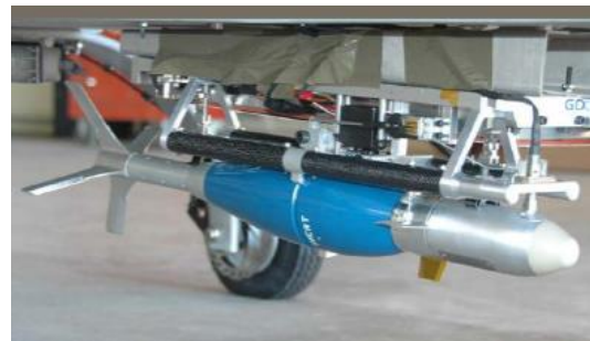
Figure 2. 81 mm Precision Air-Dropped Guided Munition (ADM) with Four Fins-General Dynamics [28]
