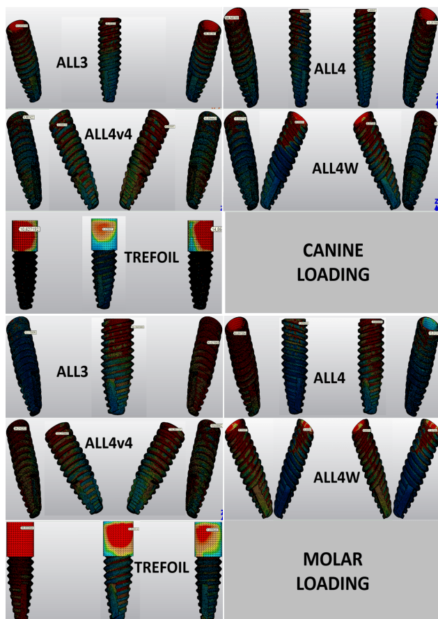
Figure 5. Von Mises Stresses on the Implants in Models Against Loadings from the Canine and Molar Regions
