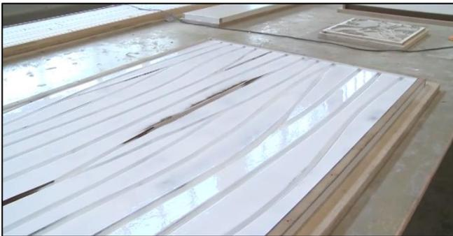
Figure 14. The model which warnished and ready for pouring silicone
