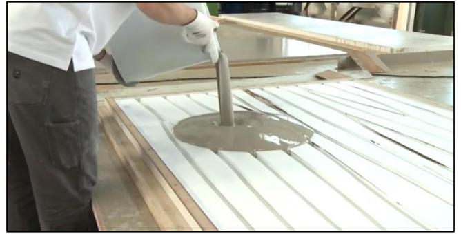
Figure 16. Pouring silicone & hardening component
