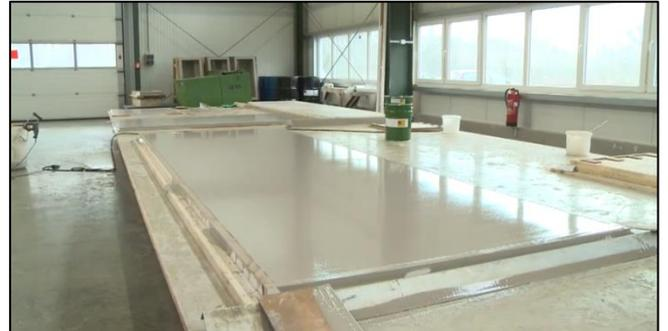
Figure 18. Silicone cast, lefted for hardening
