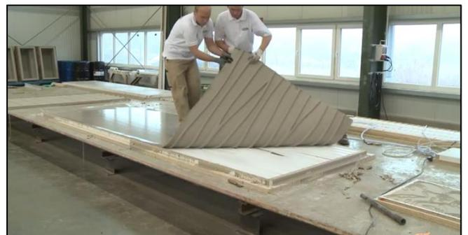
Figure 19. Removing silicone from molds
