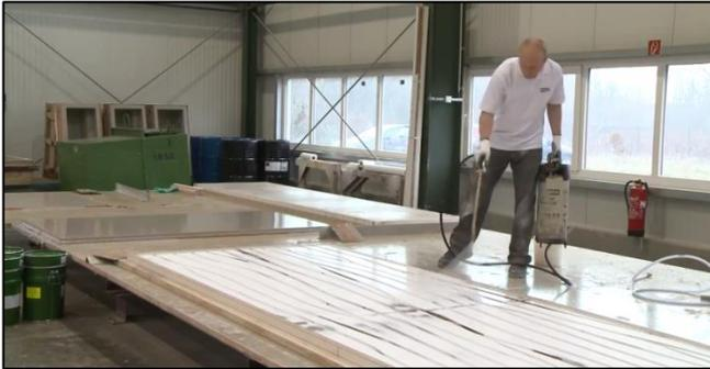
Figure 13. Warnishing mold release agent
