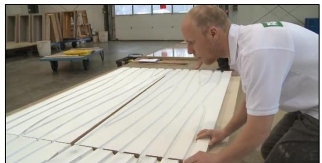
Figure 11. Interconnecting printed pattern pieces together
