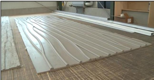
Figure 22. Silicone model, cutted and prepared for use
