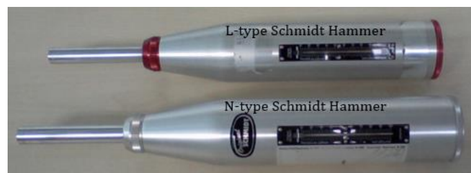
Figure 3. N-type and L-type Schmidt hammers
