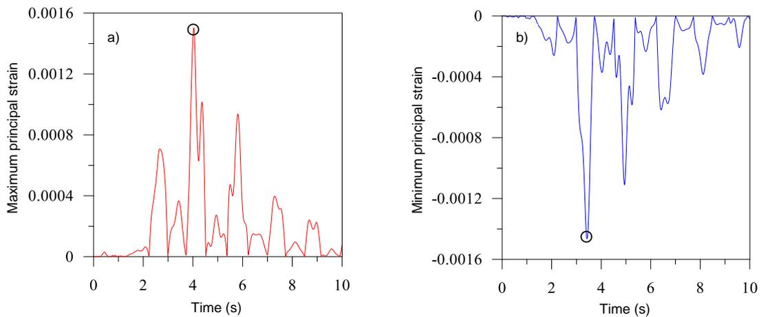
**Figure 12.** Variation of a) maximum and b) minimum principal strains with time for fixed support
