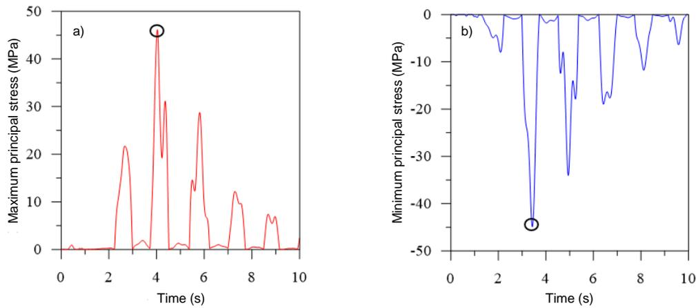
**Figure 9.** Variation of a) maximum and b) minimum principal stresses with time for fixed support
