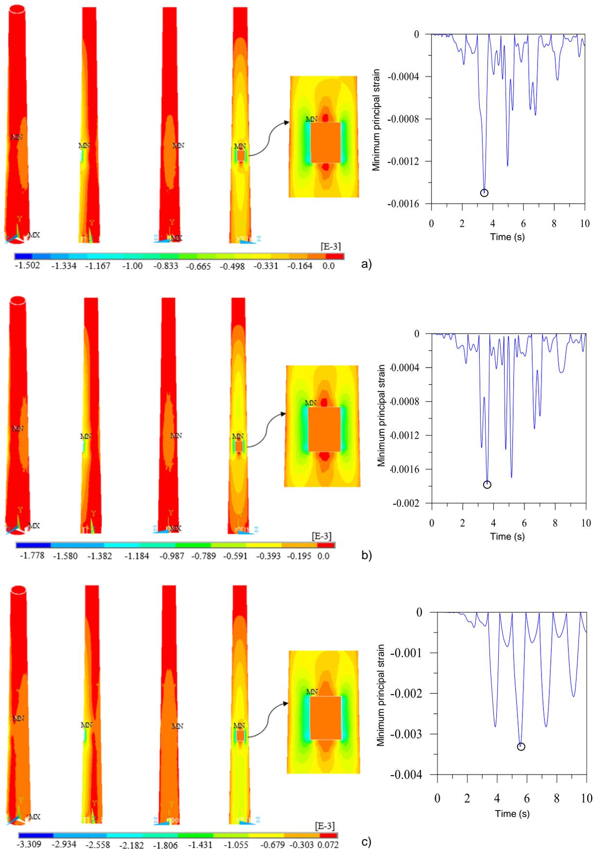
**Figure 16.** Minimum principal strain contour diagrams for FEMs containing a) hard, b) medium and c) soft soil structure interaction
