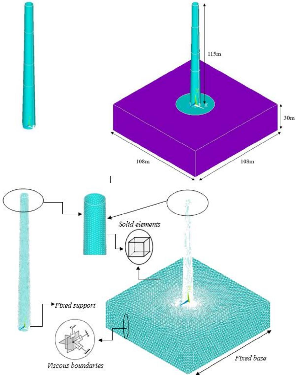
**Figure 2.** Finite element models of the chimney
