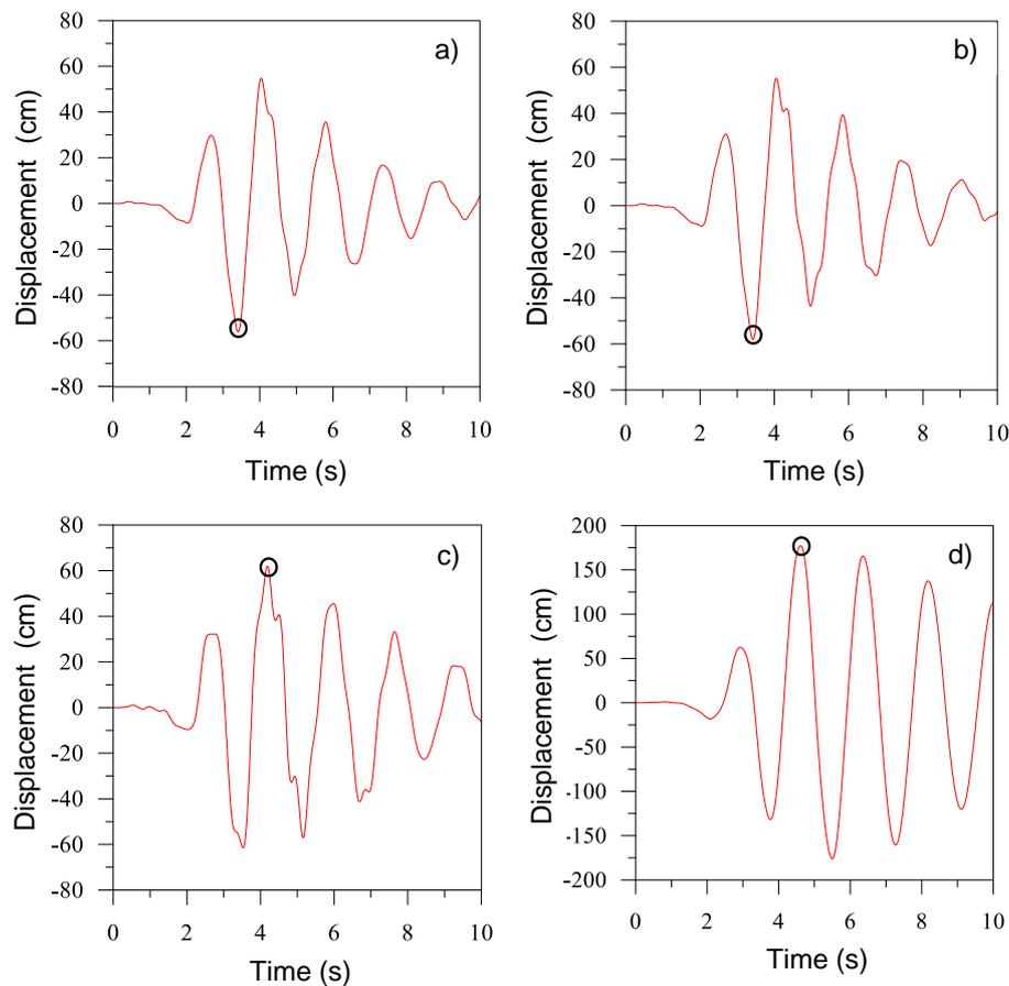
**Figure 6.** Time-dependent variation of maximum displacements for a) fixed, b) hard, c) medium and d) soft soil
