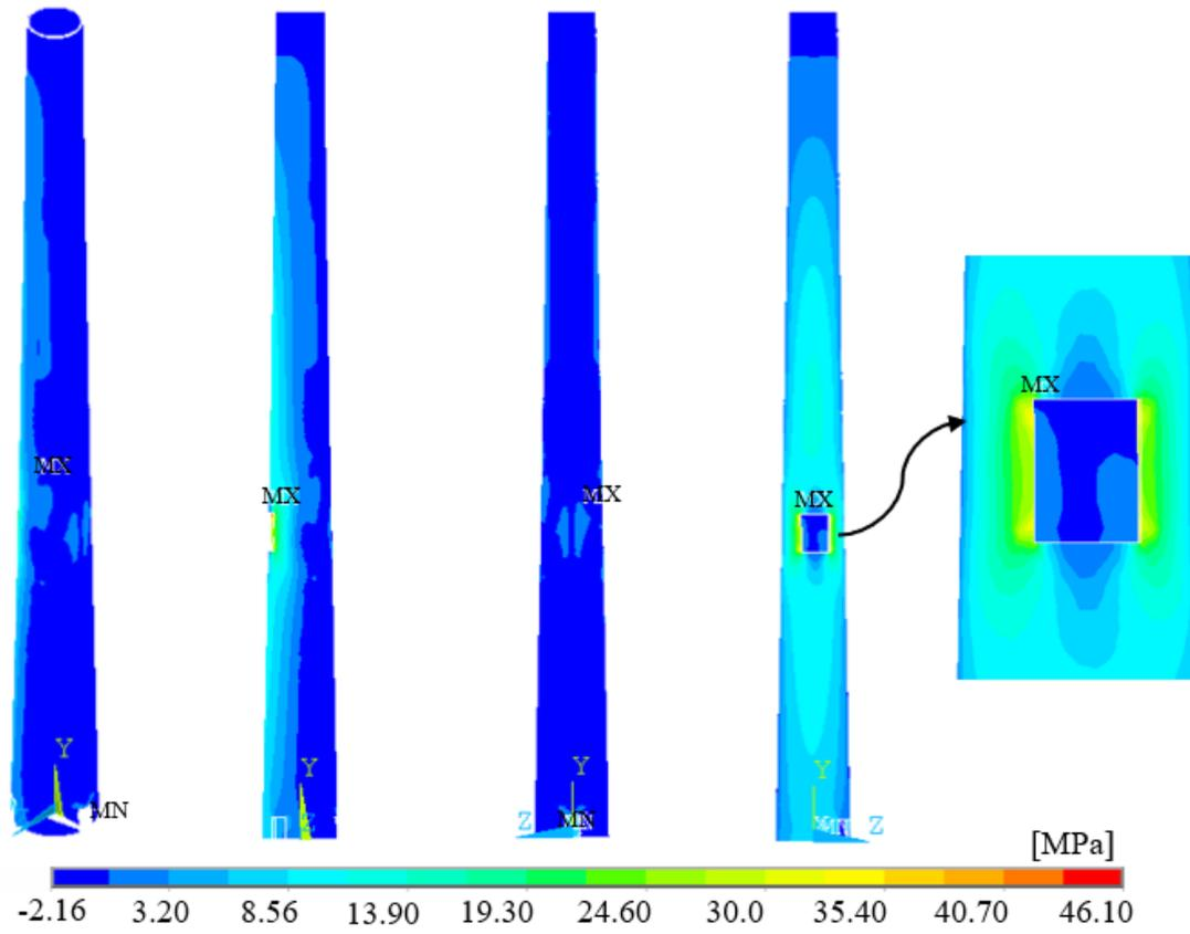
Figure 7. Maximum principal stress contour diagrams for FEM with fixed support
