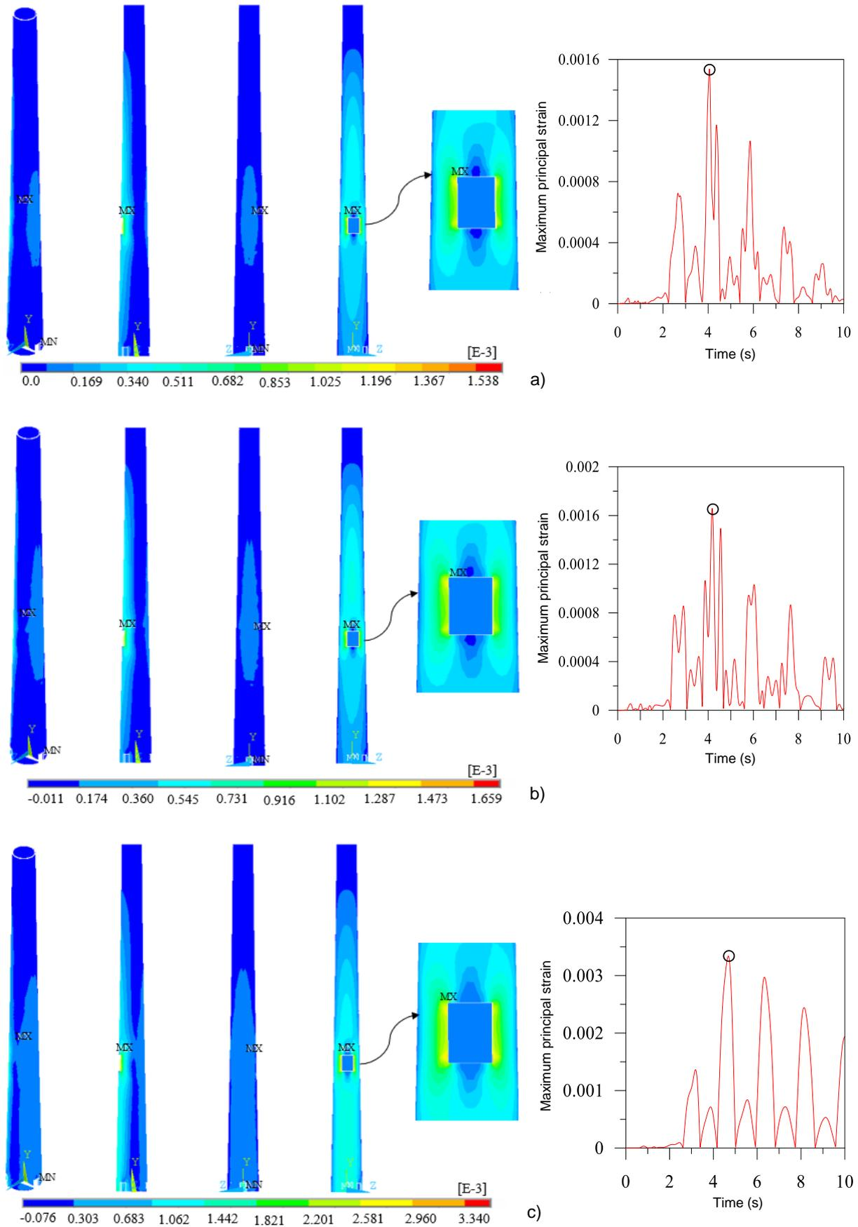
**Figure 15.** Maximum principal strain contour diagrams for FEMs containing a) hard, b) medium and c) soft soil structure interaction
