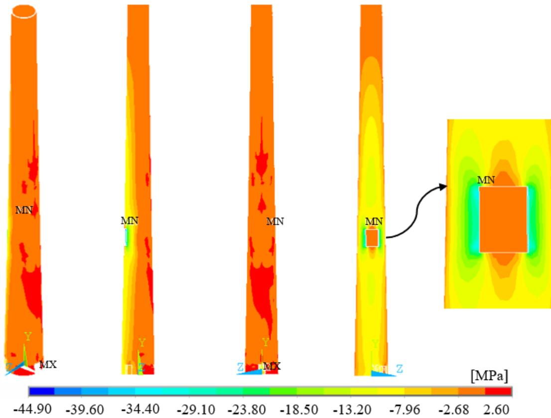
Figure 8. Minimum principal stress contour diagrams for FEM with fixed support
