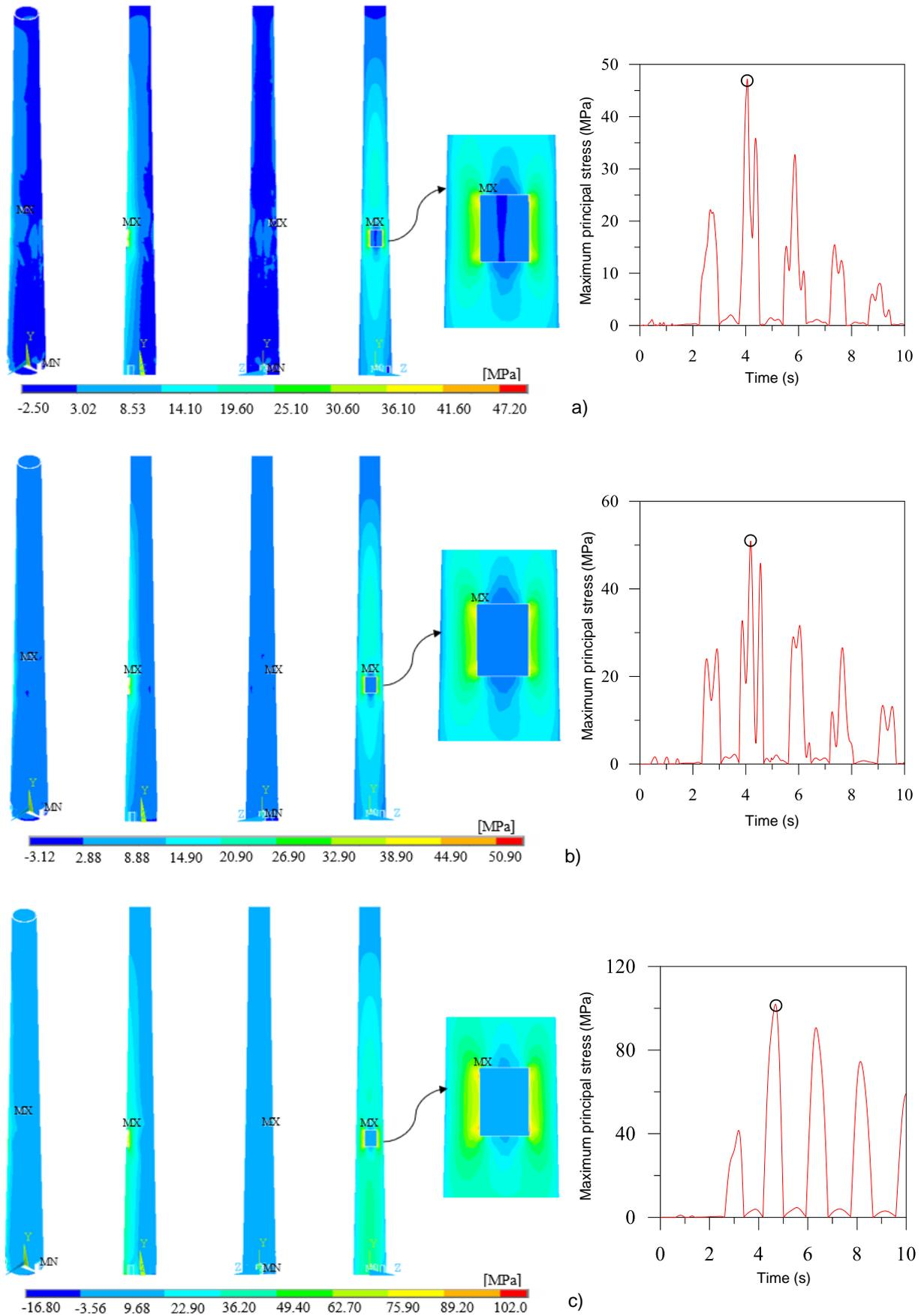
**Figure 13.** Maximum principal stress contour diagrams for FEMs containing a) hard, b) medium and c) soft soil structure interaction
