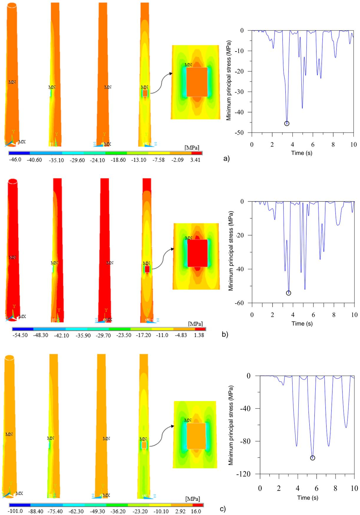
**Figure 14.** Minimum principal stress contour diagrams for FEMs containing a) hard, b) medium and c) soft soil structure interaction
