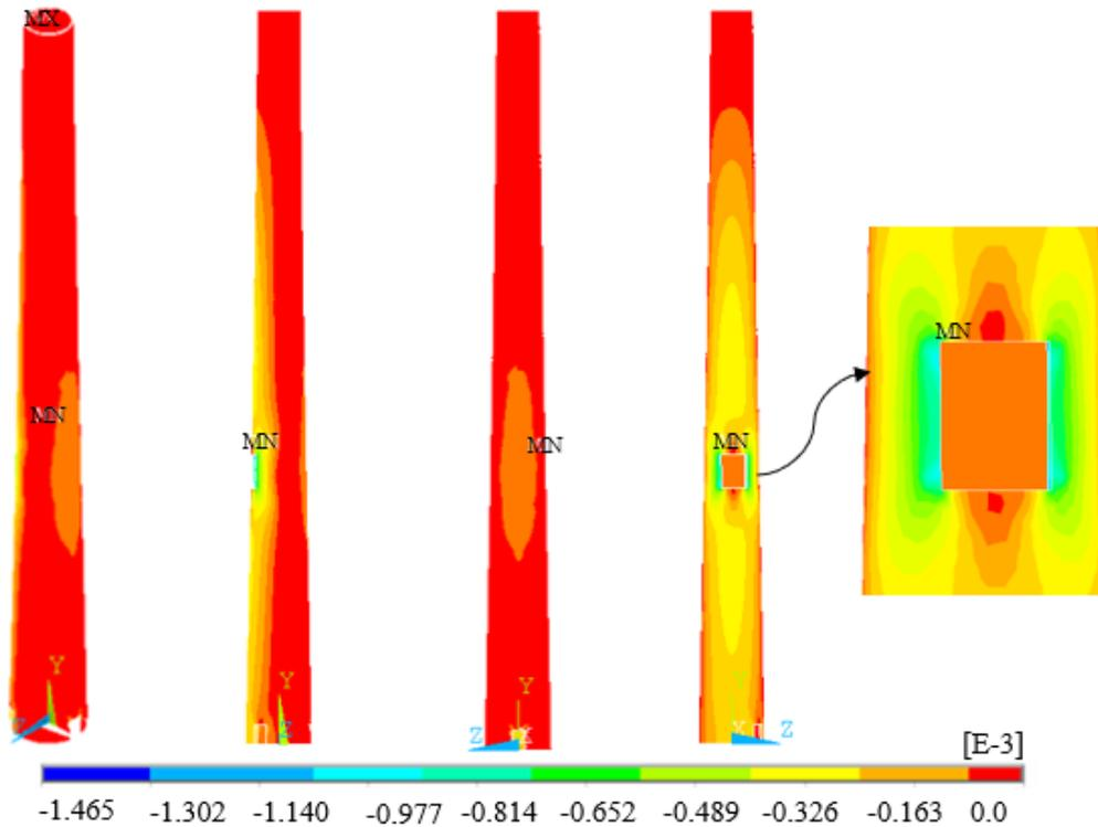
**Figure 11.** Minimum principal strain contour diagrams for FEM with fixed support
