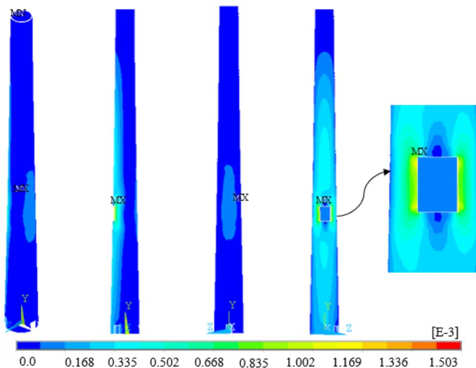
**Figure 10.** Maximum principal strain contour diagrams for FEM with fixed support
