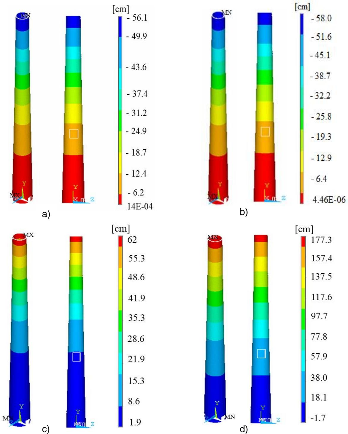
**Figure 5.** Displacement contour diagrams for a) fixed, b) hard, c) medium and d) soft soil
