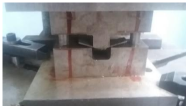
Figure 5. Modular U-bending die model
