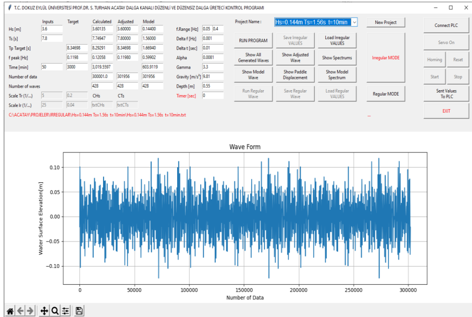
Fig. 10 The user interface of the control software.
