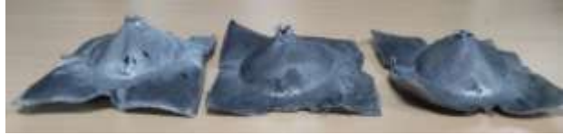
30 % Coconut shell powder filler
