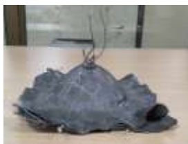
Figure 14. Images of the deformation of the composites after the impact test
