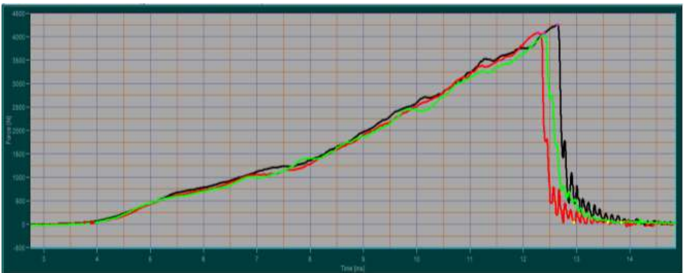
Figure 8. Energy absorption curve for 20 % of boron carbide filler added with resin
