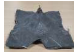
Unidirectional laid 2 layer Boron carbide filler composite
