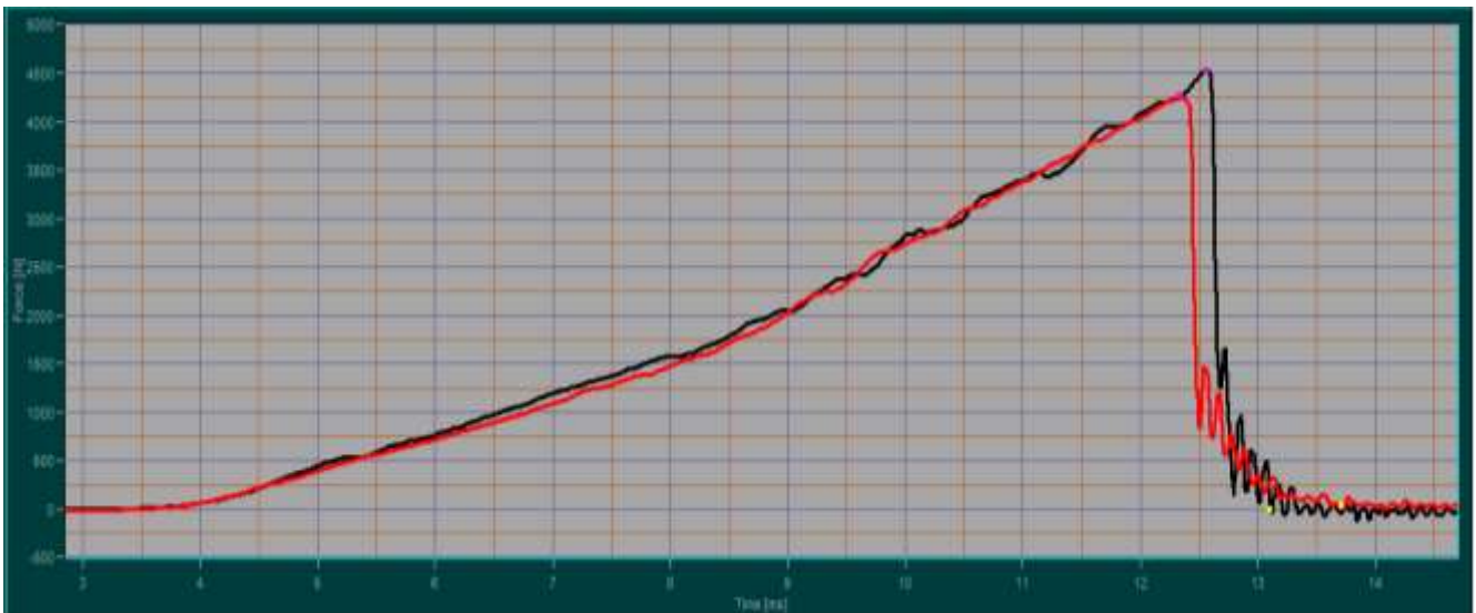
Figure 11. Energy absorption curve for 20 % of coconut shell powder filler added with resin
