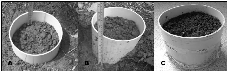
A: cylinder buried up to 15 cm deep with 5 cm edge. B: extraction of the cylinder with an undisturbed soil sample. C: cylinder prepared with canvas and mesh in its lower part.
