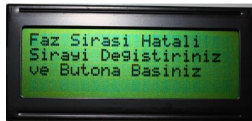
Figure 16. The state that the one of the phases is in fault.
