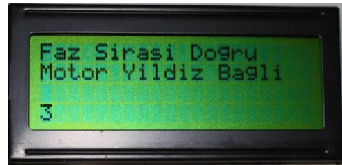
Figure 13. The state that the phase sequence is confirmed by the microcontroller and CRIM windings are wye connected.
