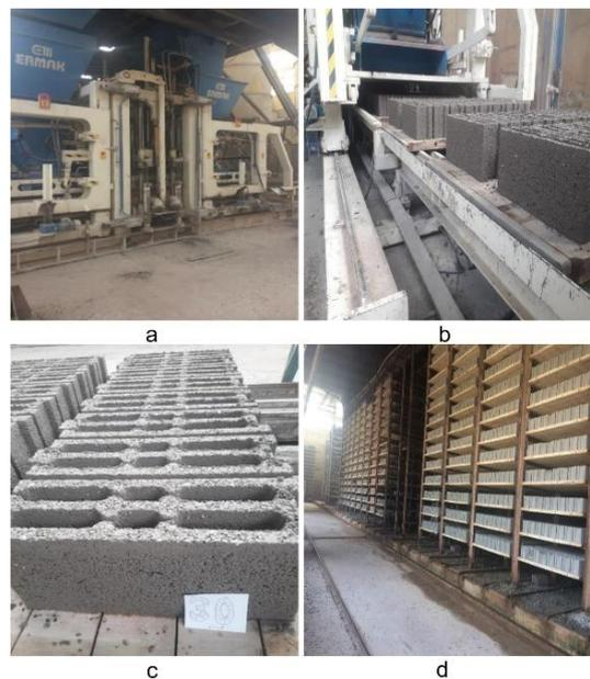
Figure 2. Production processes (a) automatic machine; (b, c) produced specimens; (d) curing
