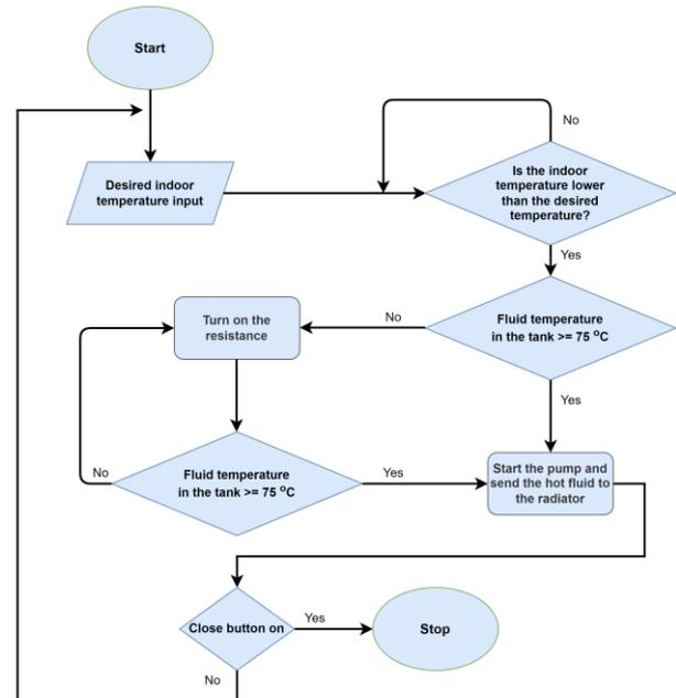
**Figure 5.** Flow chart of the hybrid heating model
