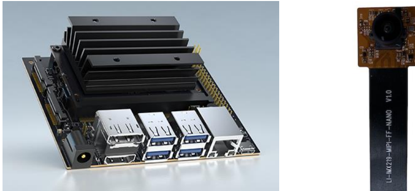
Figure 2. Nvidia Jetson Nano embedded device and CSI Camera [7->19]
