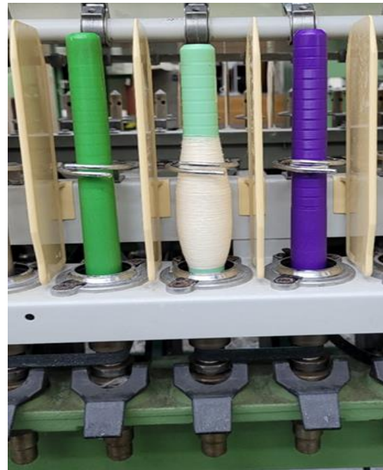
Figure 3. Spindle and Bobbin Assembly
