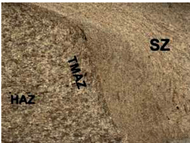
Figure 4. The transition zones for W2 welded joint.
