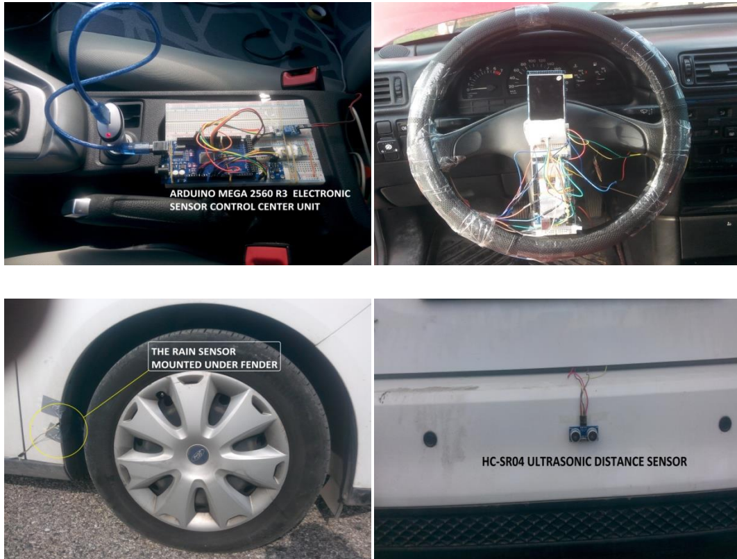
Figure 3. Mounting on the vehicle of improved vibration controlled driver warning system
