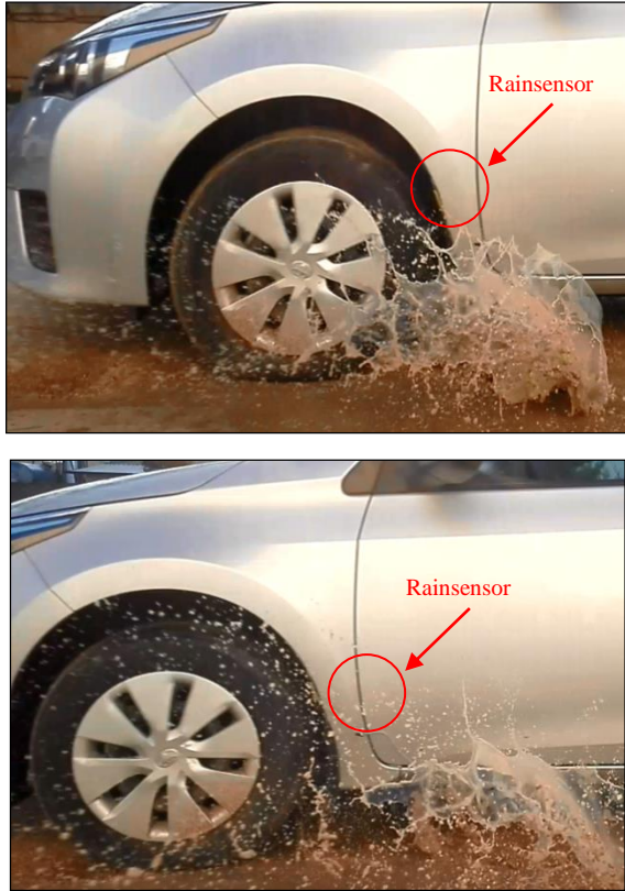
Figure 8. Driving tests for detect of the wet asphalt surface
