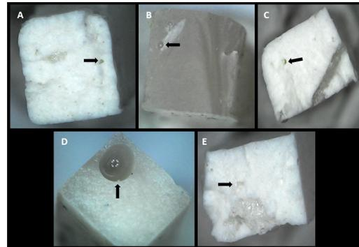
**Figure 3.** Representative light microscopy (30x) images of the fractured surfaces. **A:** ZPC-H; **B:** GILC-H; **C:** NXS-H; **D:** MXM-H and **E:** ZE-H. Black arrows represent pores at the cement's surface.
