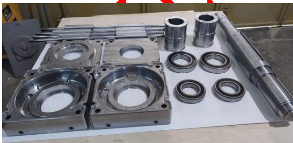
Figure 13. Produced motor components
