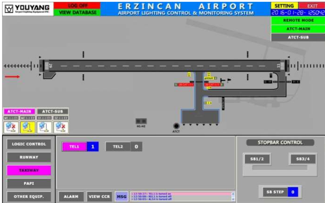
Figure 17. The commissioning of Taxiway lighting system using the Control screen
