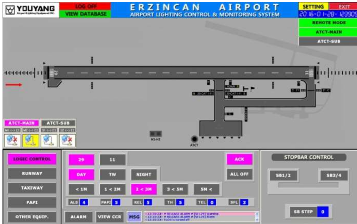
Figure 20. Using the PLC via the SCADA Runway Lighting Control Screen belong Erzincan Airport
