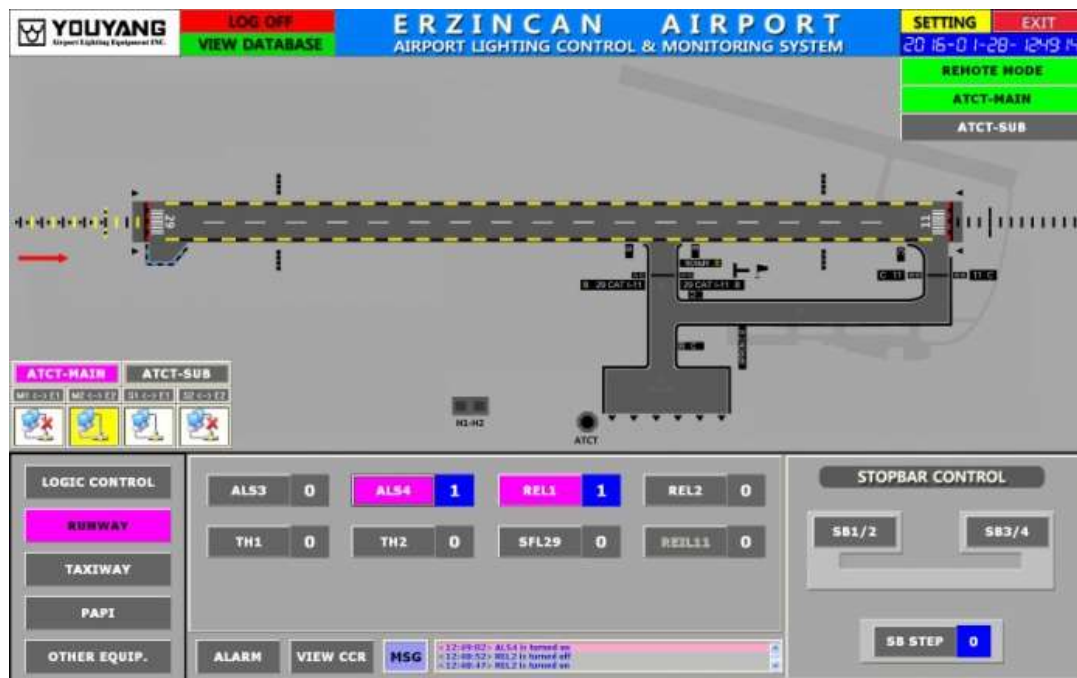
Figure 18. Commissioning of the runway edge lighting system using the control screen(yellow parts)
