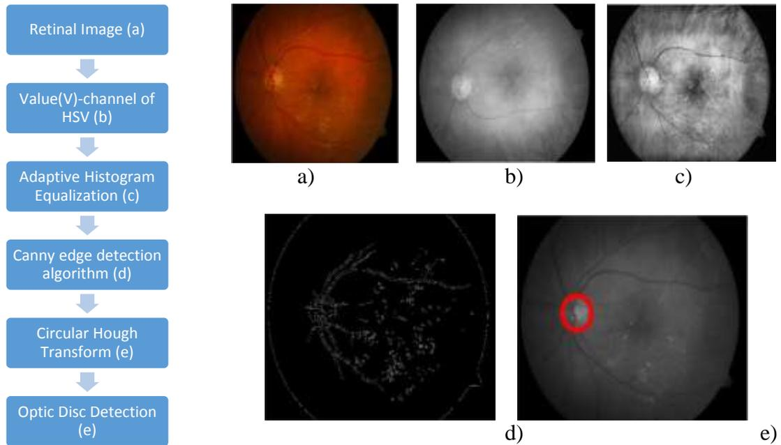
Figure 4: Optic disc detection algorithm using HSV color space and Circular Hough Transform.
