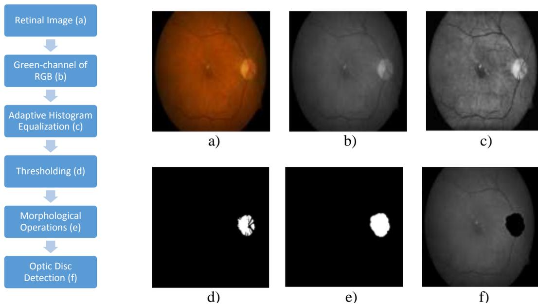
Figure 2: Optic disc detection algorithm with thresholding.
