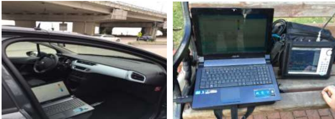
Fig.1 Measurement process with RTL2832U R820T and Anritsu S332E spectrum analyzer
