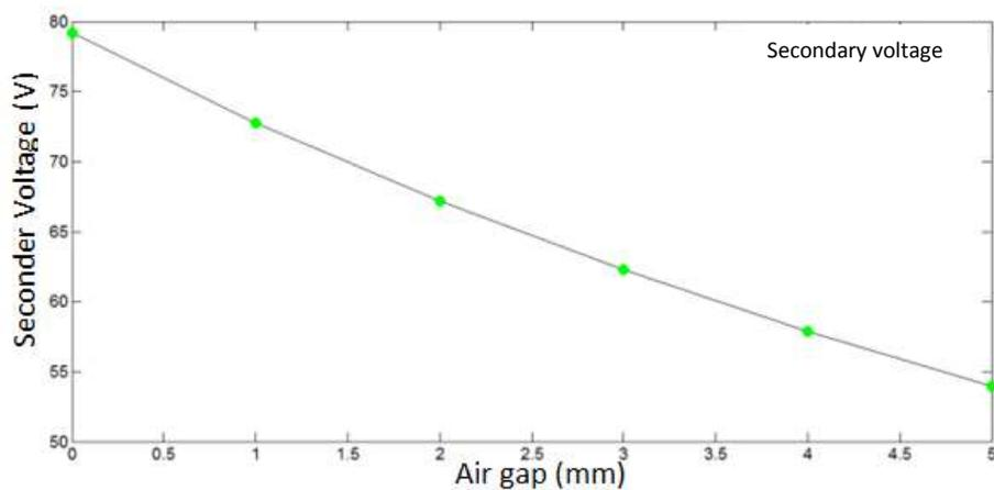
**Figure 11.** Secondary voltage ( $V_2$ ) versus airgap distance
