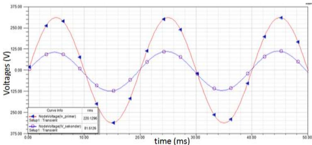
Figure 14. Voltages in no-load operation
