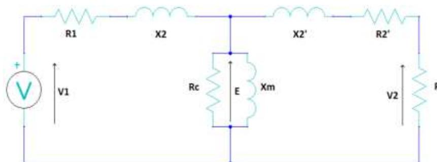
**Figure 5.** Electrical T equivalent circuit of transformer
