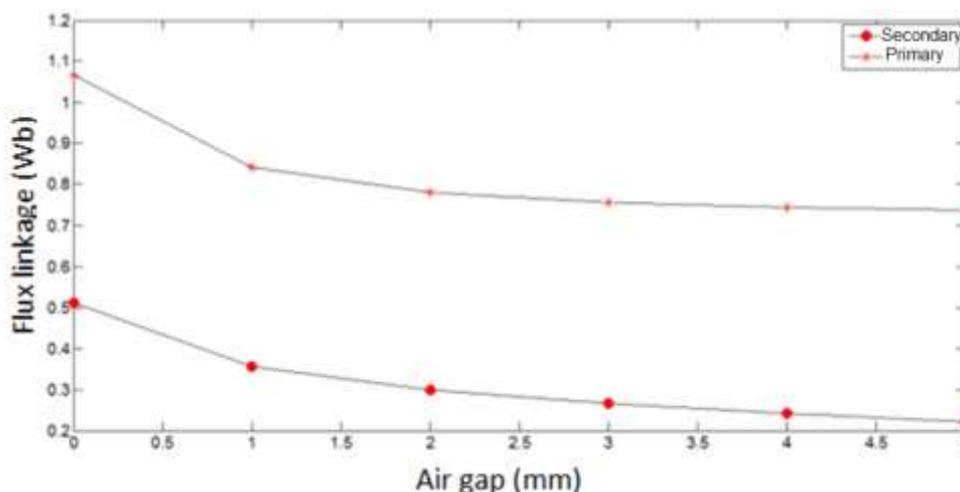
Figure9. Flux linkage versus air gap distance
