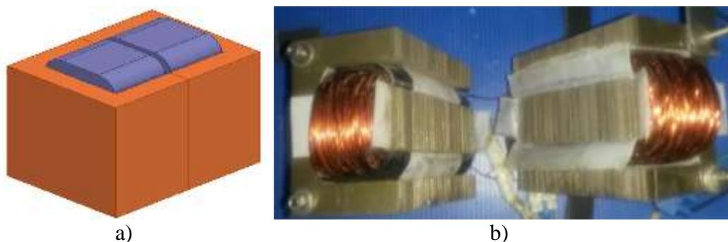
Figure 3.a) 3D design model b) transformer cores and windings
