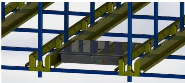
**Figure 1.** Shuttle robot
