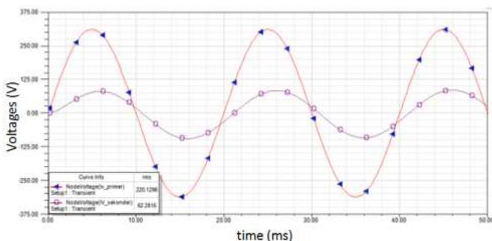
Figure 15. Voltages in full load operation
