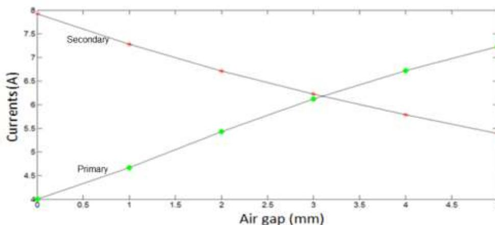
Figure 8. Current versus air gap distance
