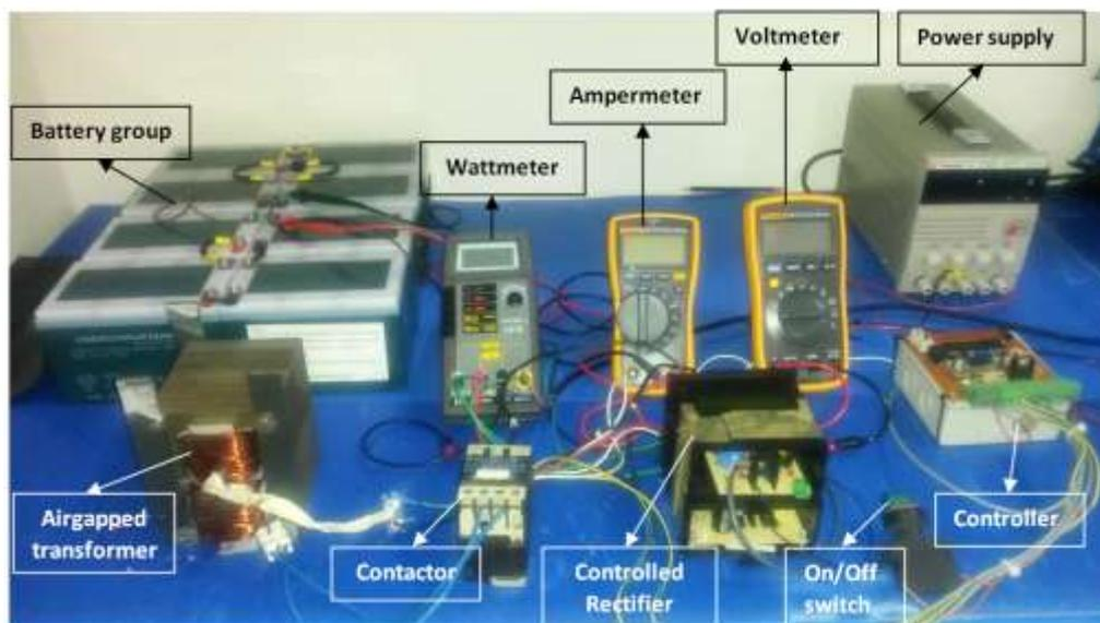
**Figure 7.** WCS experimental setup
