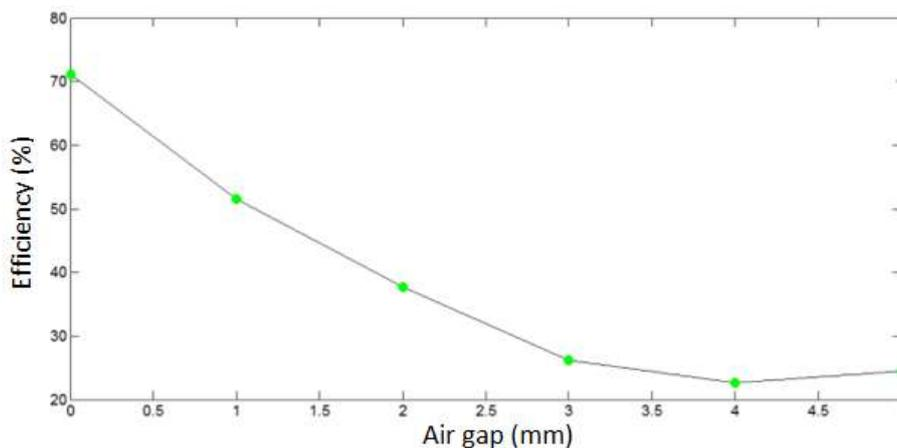
Figure 12. Efficiency versus airgap distance
