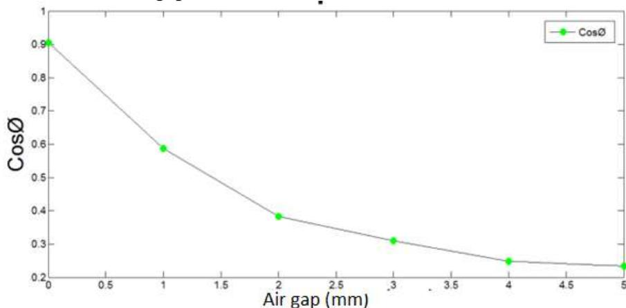
**Figure 10.** Power factor ( $\text{Cos}\phi$ ) versus airgap distance
