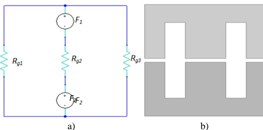
Figure 4. a) Magnetic equivalent circuit b) EE core
