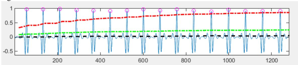
a) QRS points detected on ECG signal filtered through Pan-Tompkins algorithm.
