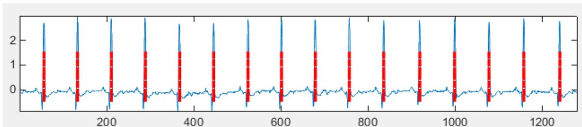
b) QRS points shown on Standard ECG signal.
