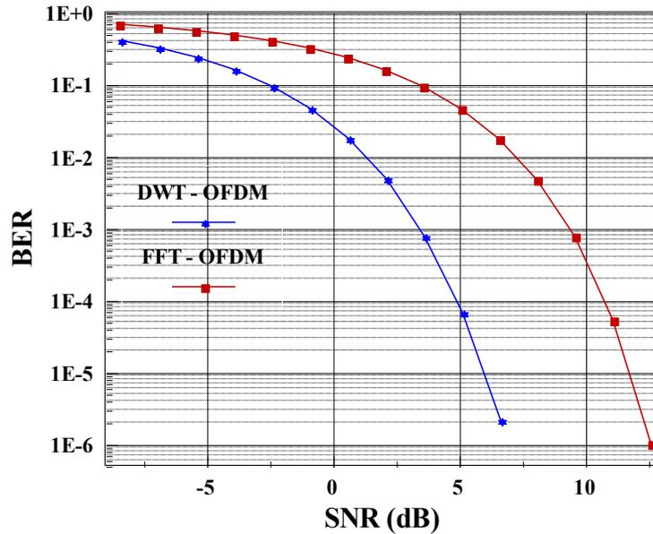
**Figure 4.** Comparison BER versus SNR performances of conventional FFT-OFDM and DWT-OFDM systems in AWGN channel for 4-QAM.
