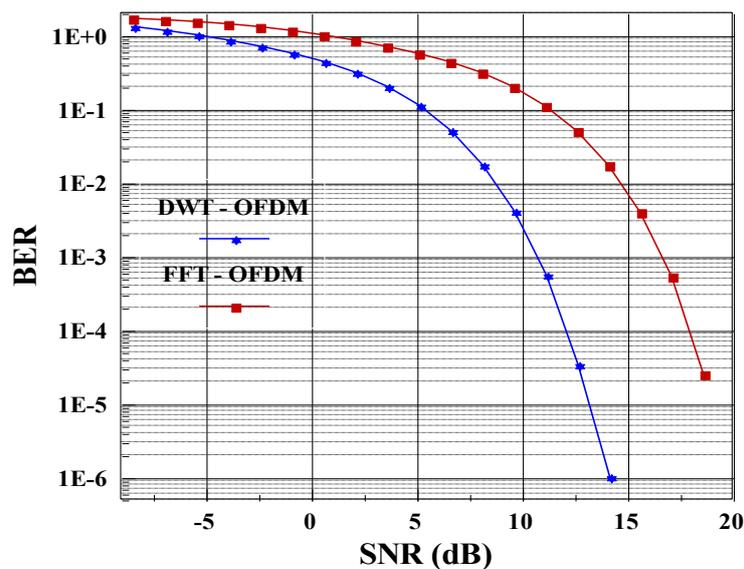
**Figure 5.** Comparison BER versus SNR performances of conventional FFT-OFDM and DWT-OFDM systems in AWGN channel for 16-QAM.
