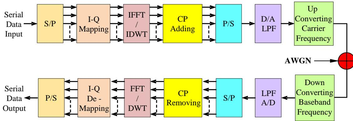
Figure 1. The block diagram of FFT/DWT – OFDM system [17, 18].
