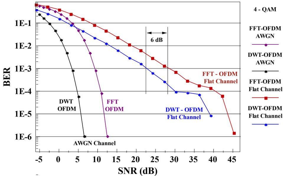
**Figure 7.** Comparison BER versus SNR performances of conventional FFT-OFDM and DWT-OFDM systems in AWGN channel with AWGN and frequency flat Rayleigh fading channel for 4-QAM.
