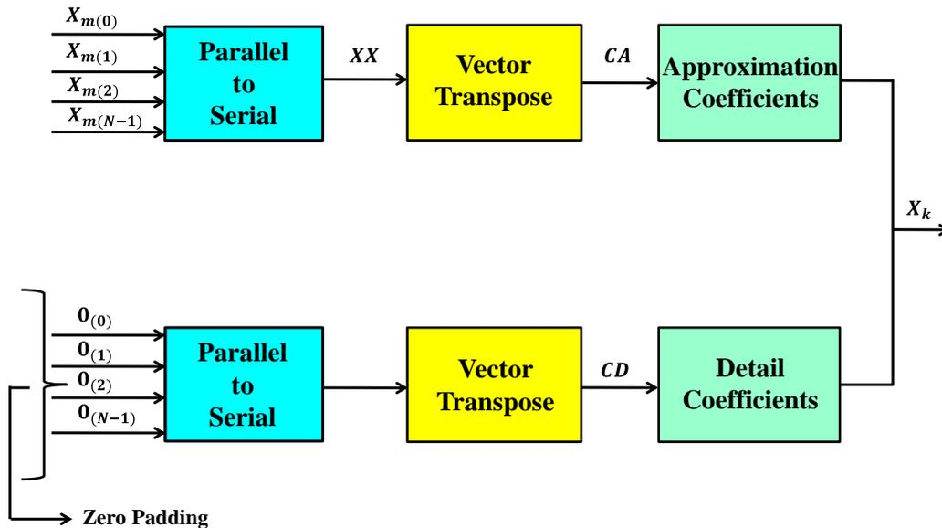
Figure 2. The block diagram of DWT – OFDM transmitter system [17, 18].
