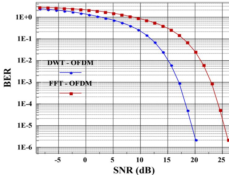
**Figure 6.** Comparison BER versus SNR performances of conventional FFT-OFDM and DWT-OFDM systems in AWGN channel for 64-QAM.
