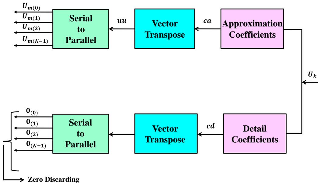
**Figure 3.** The block diagram of DWT – OFDM receiver system [17, 18].
