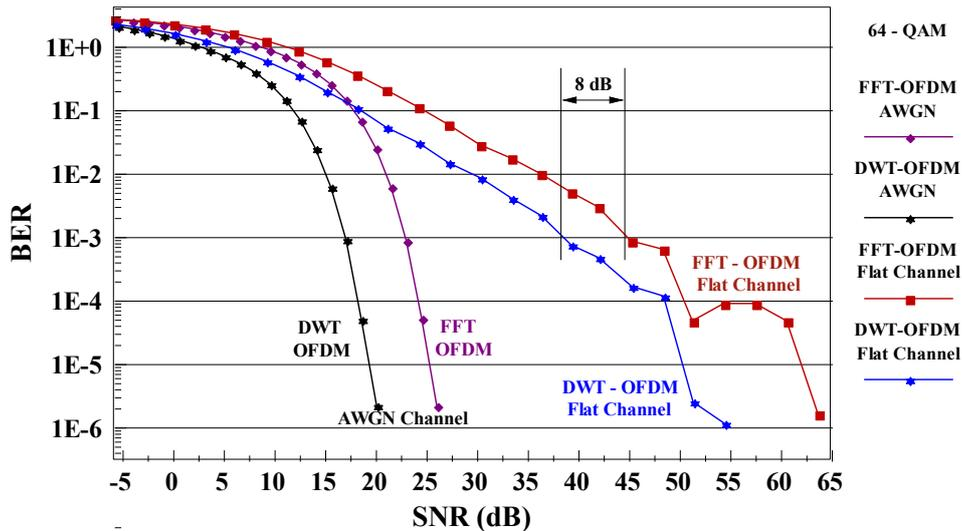
**Figure 9.** Comparison BER versus SNR performances of conventional FFT-OFDM and DWT-OFDM systems in AWGN channel with AWGN and frequency flat Rayleigh fading channel for 64-QAM.
