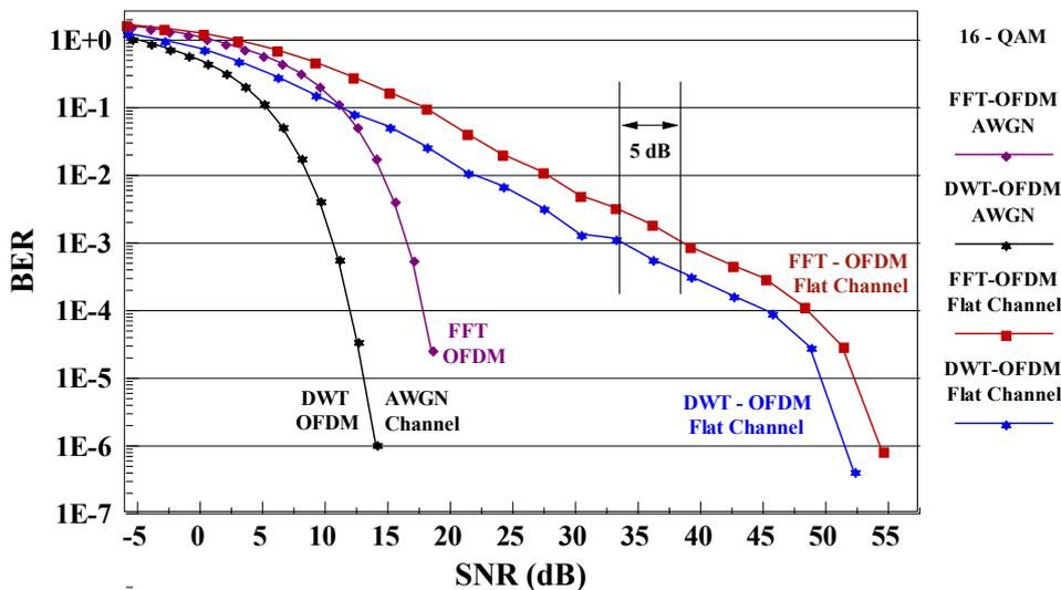
**Figure 8.** Comparison BER versus SNR performances of conventional FFT-OFDM and DWT-OFDM systems in AWGN channel with AWGN and frequency flat Rayleigh fading channel for 16-QAM.
