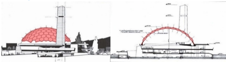
Figure 3. Terzi Baba Mosque dome and the designed hexagonal top cover section and view (URL-1).
