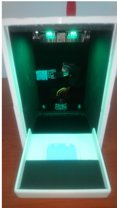
Figure 2. The developed system ready to emit green light to the half of the active surface of the PSP. The front door is opened for visualization of the electronic units in the photo.
