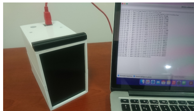
Figure 1. Sensor readings are monitored through the serial port.
