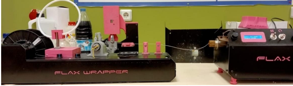
Figure 3. Flax brand name laboratory scale extruder and filament wrapper machine
