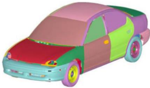
Fig. 5. The detail of FE model of 1996 Dodge Neon. [13]
