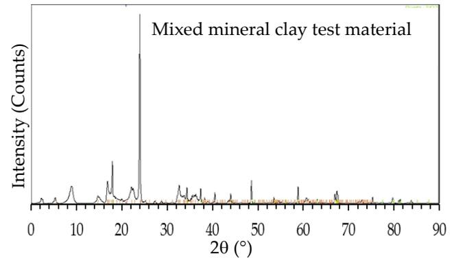
Figure 1. XRD pattern of the MMC test material.
