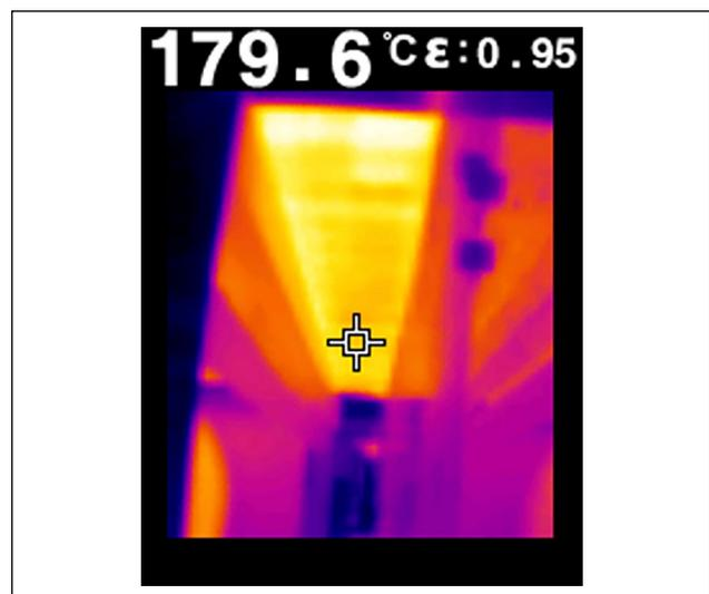
**Figure 3.** Thermographic images of the top baking plate during operation shows 179.6°C, the emissivity adjusted to measure with 0.95.
