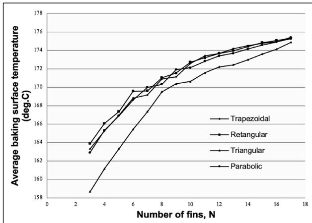
**Figure 10.** Average baking surface temperature of the plate finned with variable number of trapezoidal, triangular parabolic and rectangular fins.
