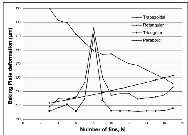
**Figure 12.** Maximum deformation  $\delta$  of the baking plate due baking pressure caused by the steam generation from the baking dough.
