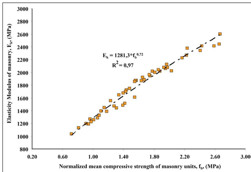
Figure 16. The elasticity modulus of the masonry section.
