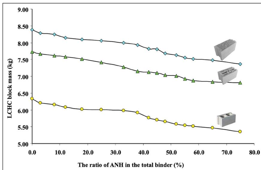
Figure 9. Effect of ANH replacement level on the mass of LCHC block specimens.
