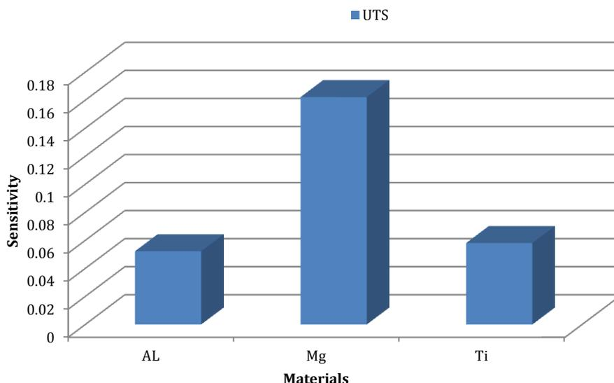
Fig. 3: Sensitivity of the materials on tensile strength
