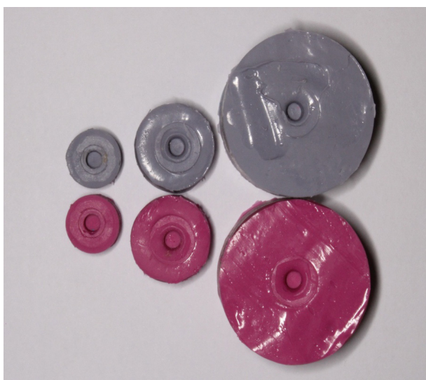
Figure 4. Polyvinyl siloxane samples with a space at the center for dental material: High-viscosity PVS (Grey) and Medium-viscosity PVS (Pink)
