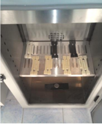
Figure 1. UV aging of PP/ZnB polymer composites
