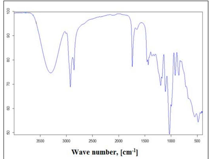
**Figure 3.** FT-IR spectrum of the grinding aid
