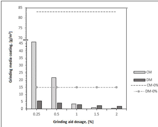
Figure 7. Grinding media coating of calcitic and dolomitic marble
