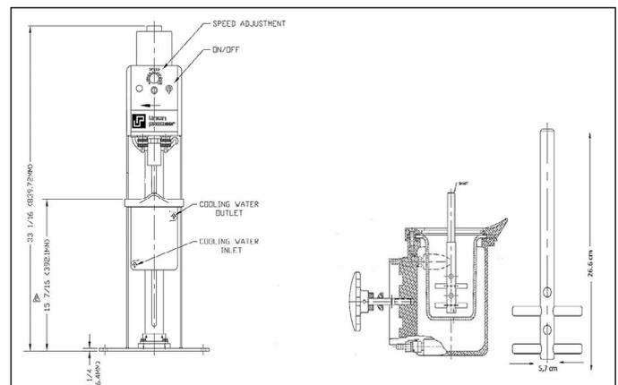
**Figure 4.** Laboratory-scale vertical stirred ball mill
