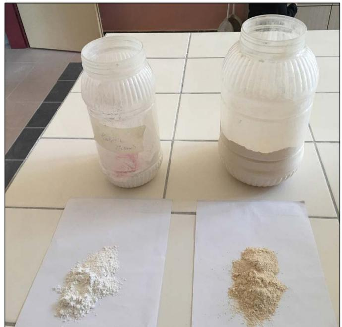
**Figure 1.** The appearance of Afyon white (calcitic) marble and Aydın yellow (dolomitic) marble dust
