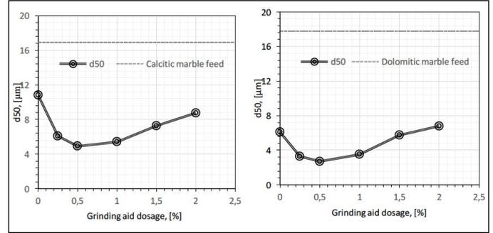
**Figure 5.** Influence of the grinding aid concentration on the  $d_{50}$  size
