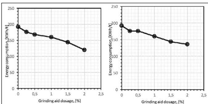
Figure 8. Energy consumption of calcitic and dolomitic marble
