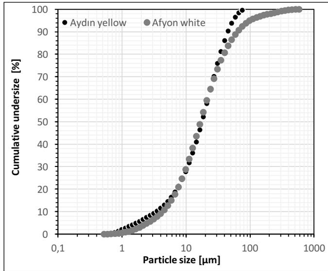
**Figure 2.** Particle size analysis of the samples used in the experiments
