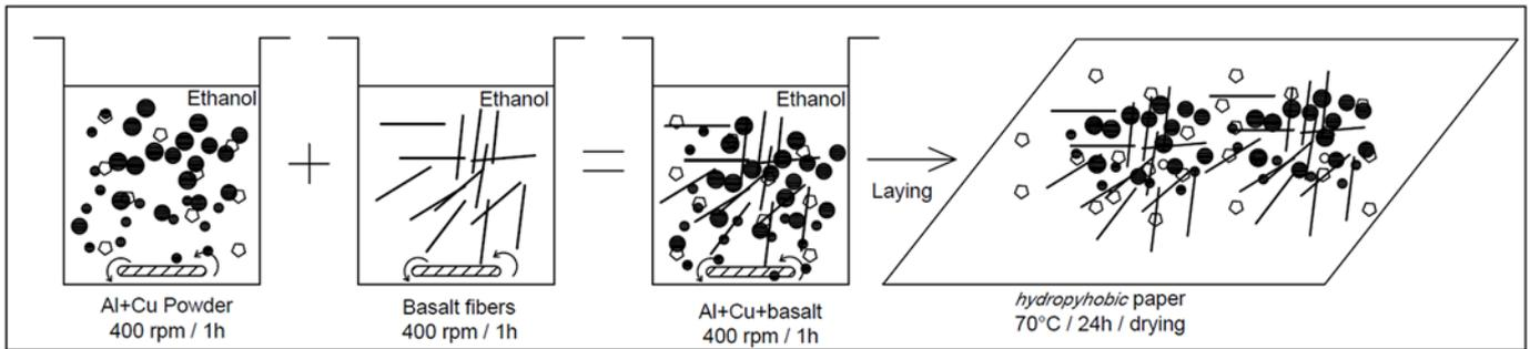
Fig. 2. Mixing process
