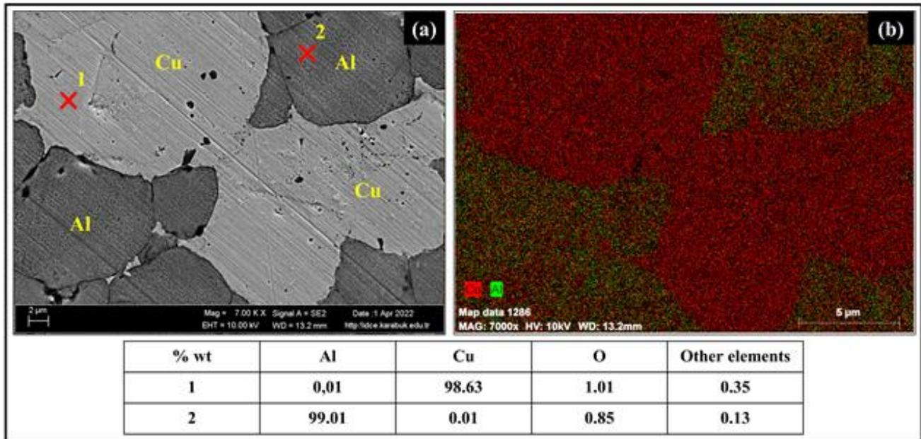
Fig. 3. SEM image (a) and EDX analyzes (b) of AlCu specimen
