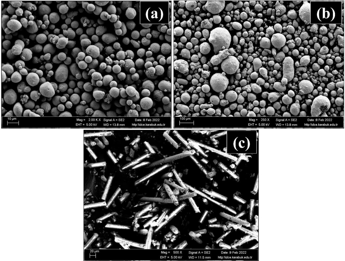
Fig. 1. SEM images of the powders and fiber reinforcement (a) Al, (b) Cu, and (c) Basalt fiber
