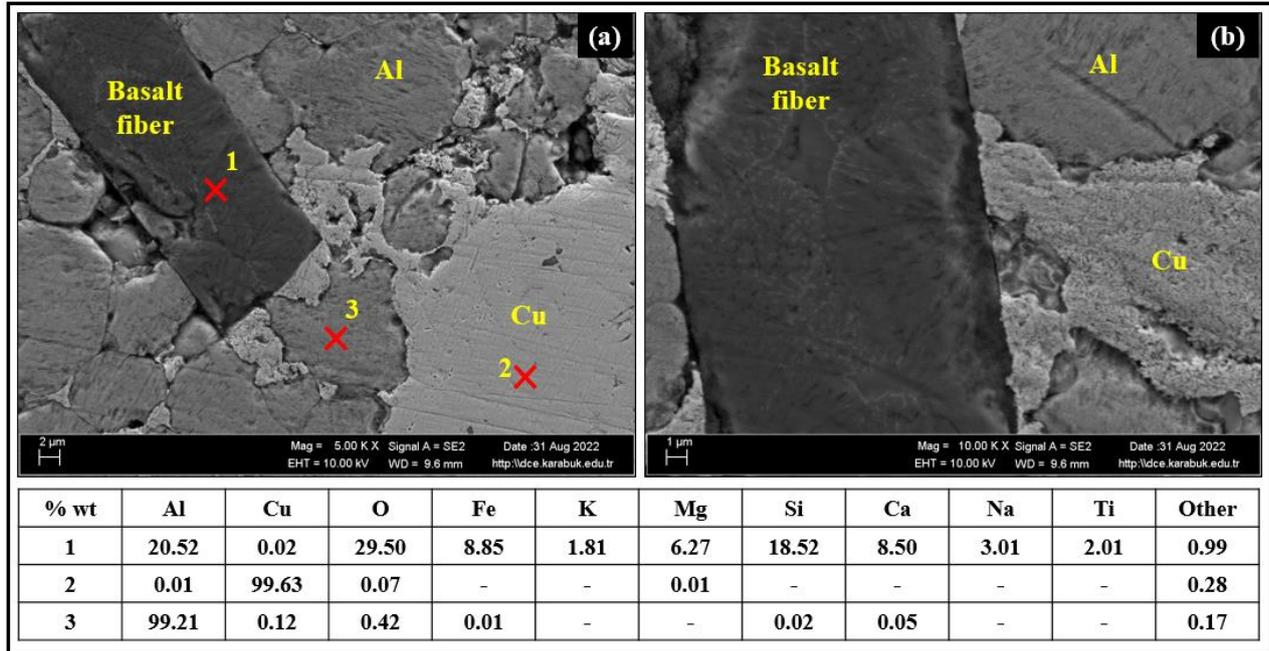
Fig. 4. SEM images of AlCuBsl specimen (a-b) high-low magnification
