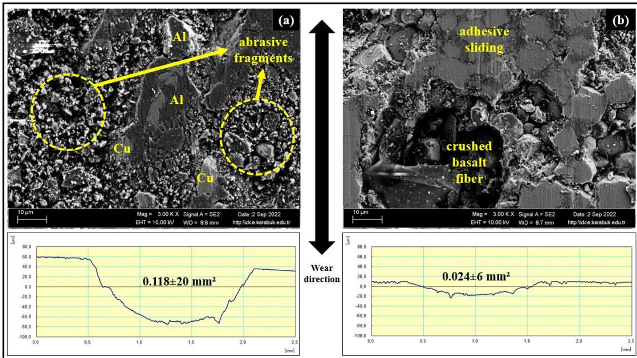
Fig. 5. Worn surfaces SEM images (a) AlCu, (b) AlCuBsl and profilometer measurements
