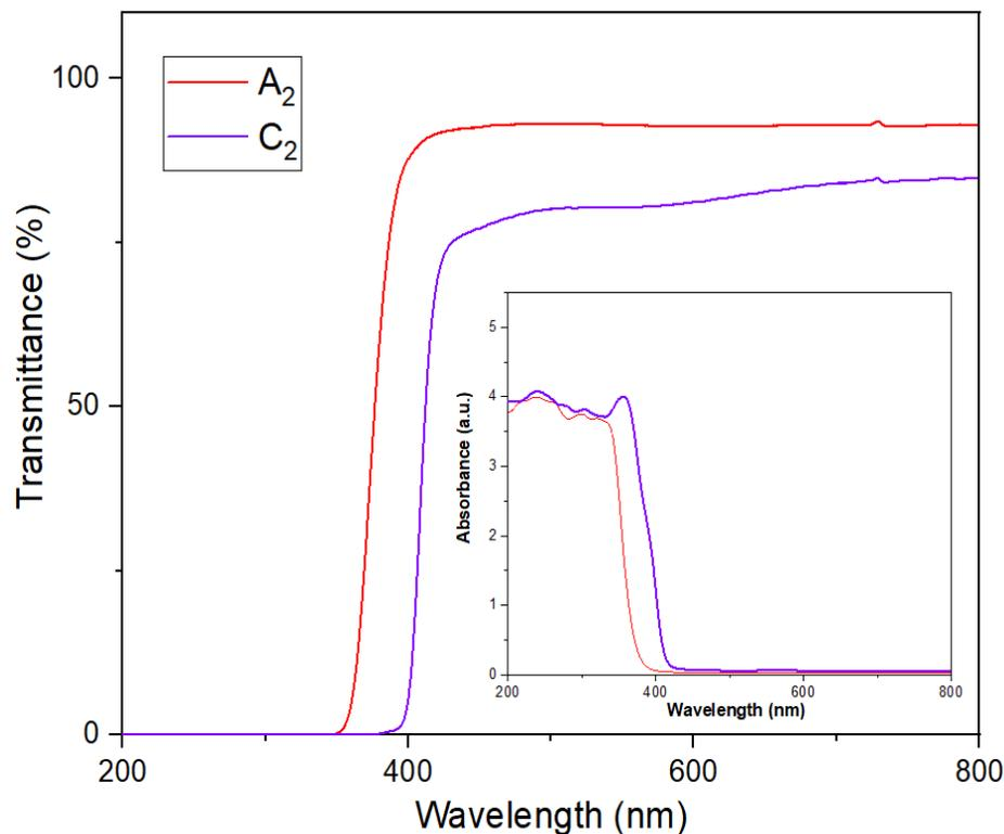
**Figure 2.** Transmittance and Absorbance Spectra of Multifocal (A<sub>2</sub>, C<sub>2</sub>) Organic Lens Samples
