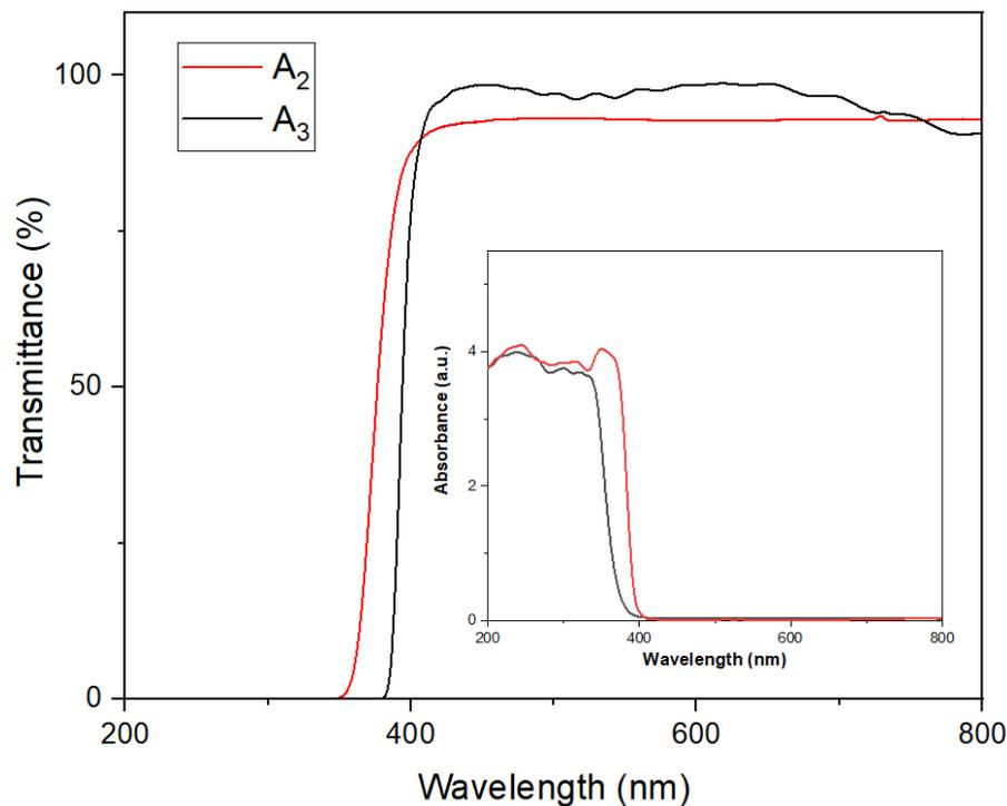
**Figure 3.** Transmittance and Absorbance Spectra of UV Protective Coated (A<sub>2</sub>, A<sub>3</sub>) Organic Lens Samples
