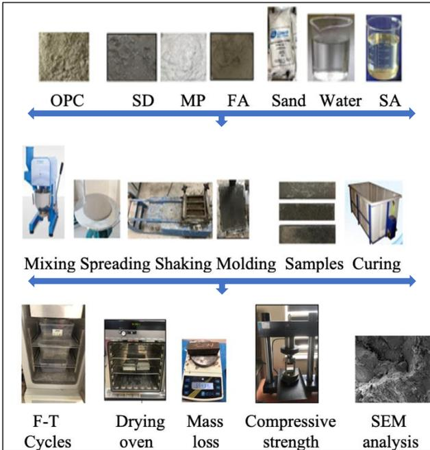
Figure 1. The schematic view of the testing stages
