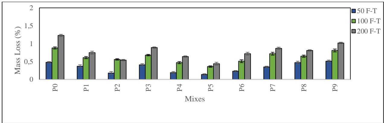
**Figure 2.** Variation of mass loss of control and FA, SF and MP blended cement mortar specimens
