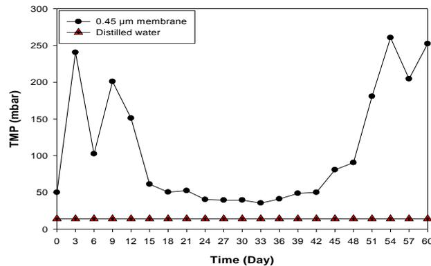
Fig.5: Pressure measurement of the real membrane through MBR operation.
