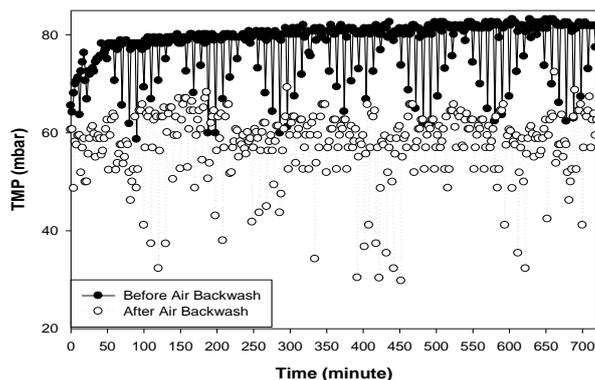
Fig. 7: Pressure values before and after air backwash.
