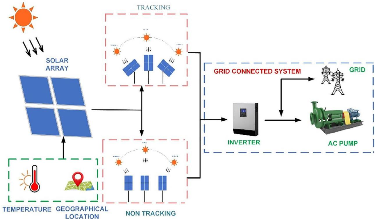
Figure 1: Solar Pumping System Configuration [11]
