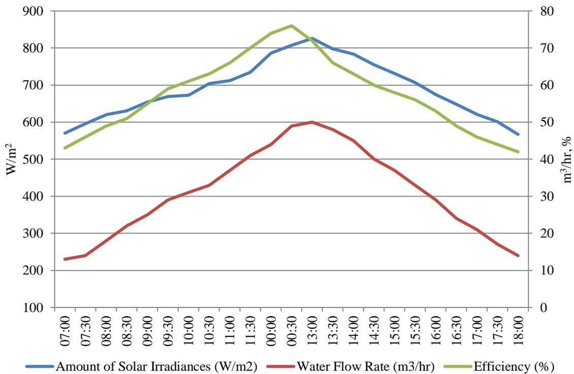
Figure 5: Performance of Fixed Solar Pumping System for Cloudy Day
